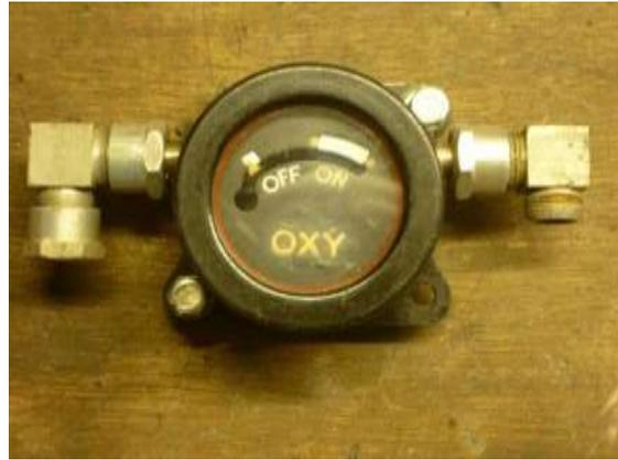
The indicator fits onto the left support tube, with oxygen pipes going through the two holes visible below it. There was damage to the turret ring where the bare aluminium can be seen which appears to be from a support tube suffering impact.
