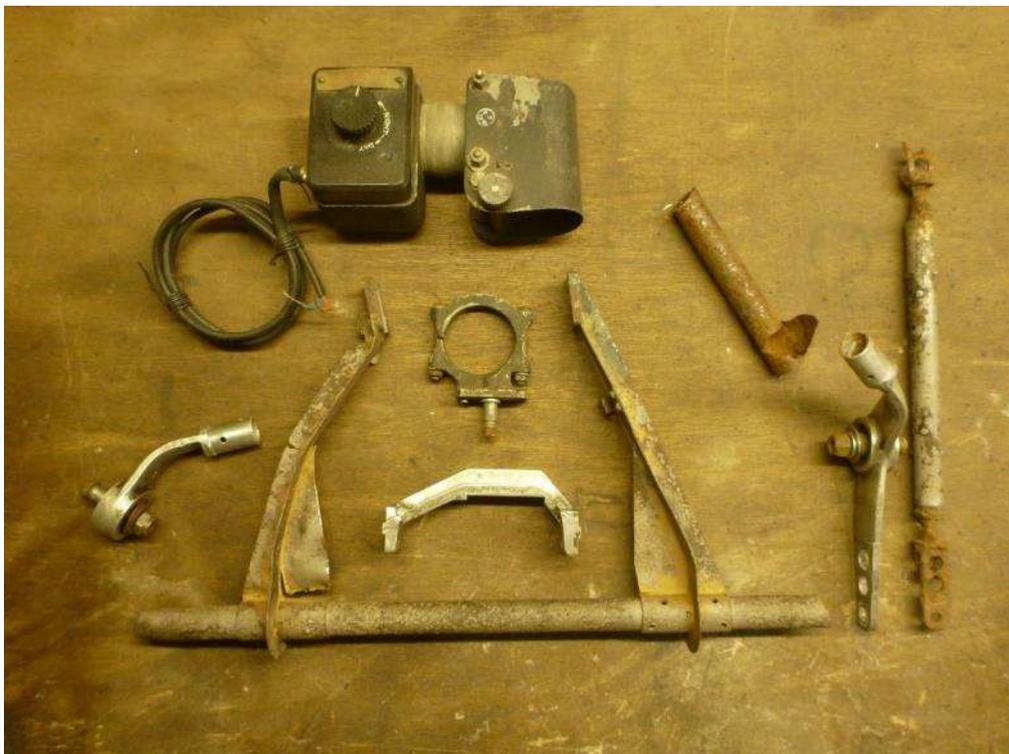
Although the original alloy castings were in very good condition, the actual radius arm which is made of steel was only really suitable to use for a pattern. The MkIIIA reflector gunsight came from a well known on-line auction site. A day or two of light hearted tin bashing produced a passable radius arm, which was bolted in to check it for size, angles and the like.
