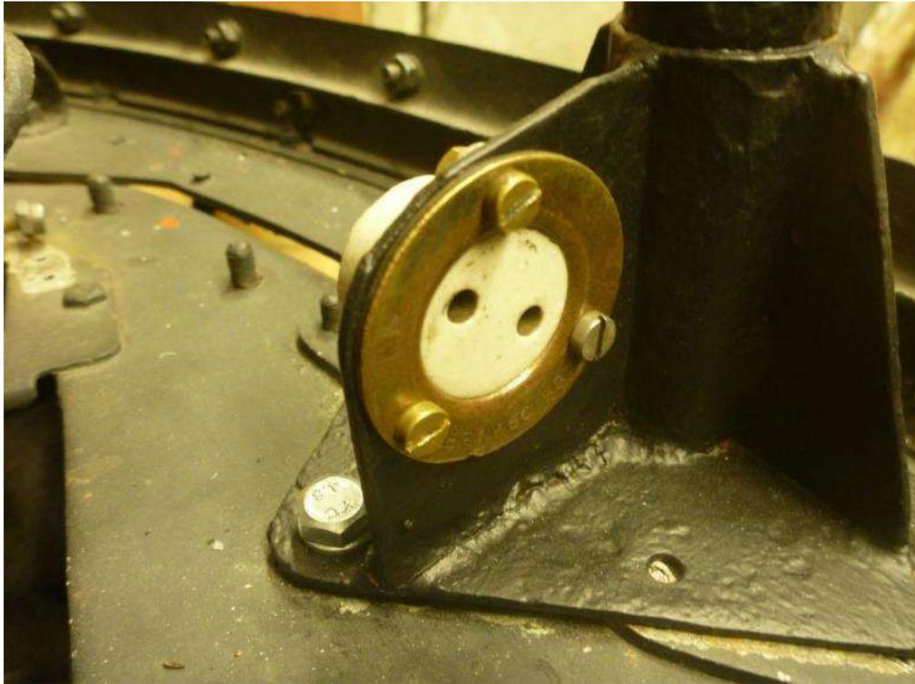
As mentioned earlier, the support tubes also provide the mounting points for the gun sight radius arm and, therefore, the gun sight. This assembly made the obvious choice for the next project but there was a lot of work to get this into a reasonable state.
