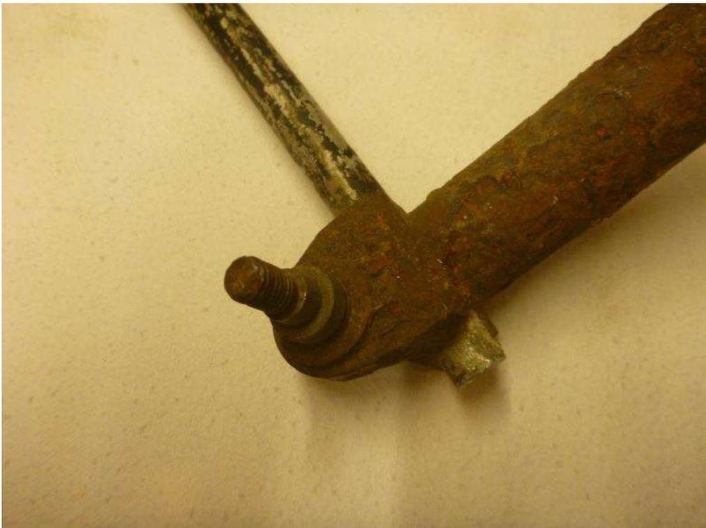
The rust soon gave up the fight and there was a small amount of welding to do to get these supports back into action. Once done it was a relatively simple task to bolt them to the turret ring and side frames.
