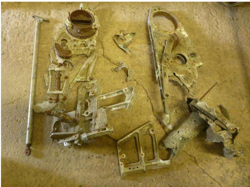
Although very badly corroded, the alloy casting is perfectly good enough to use and the steel plunger can either be restored or used as a pattern. All ways round getting this bracket provides the last major missing item (except x2 Browning 303s). Fitting it at this point might be considerably harder than I had previously predicted, however.
